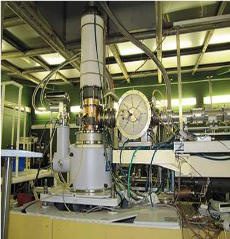
Gyrotron test facility for international project ITER
